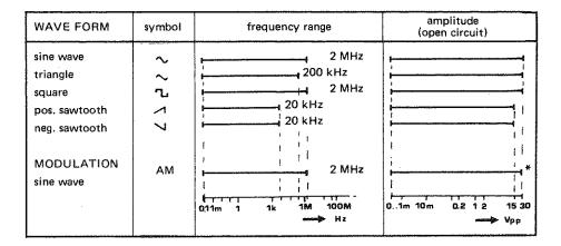
\*) carrier amplitude reduced by 6 dB
